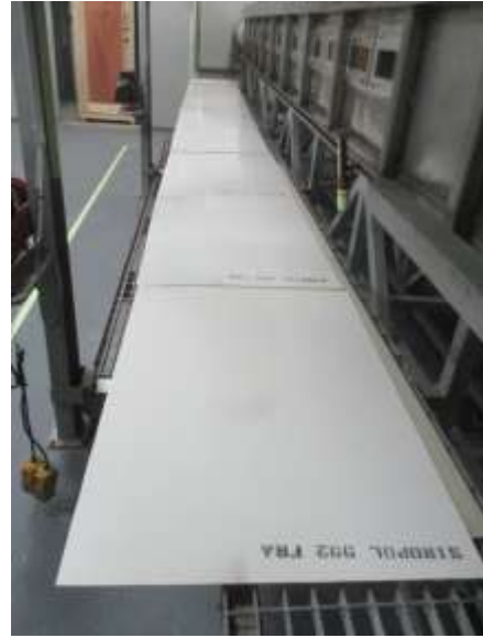
Photo 2: Specimen before the test. (Fire Side)
