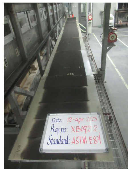
Photo 4: Specimen after the test. (As seen from the exhaust end)
